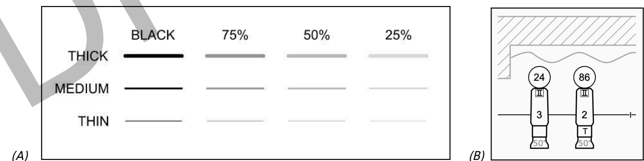
(Figure 2.3.3.0.1: (A) Different line weights and grayscale/opacity. (B) Use of grayscale lines for performance venue architectural lines to focus visual attention on lighting devices.)
